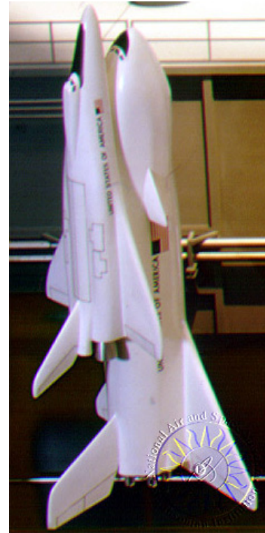
Figure 10. Model of late 1960's Rockwell two-stage fully-reusable space access system (courtesy of the National Air and Space Museum).
