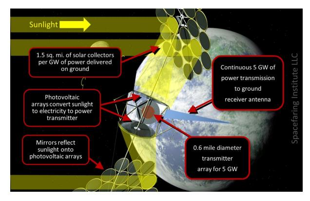
Space solar power (SSP) places the solar power systems into Earth orbit, most likely in geostationary Earth orbit (GEO) where communication satellites are located. This enables the generated electrical power to be continuously transmitted to ground receiving stations located in the United States. The ground receiving stations would function as baseload power plants providing electrical power almost continuously throughout the year.
